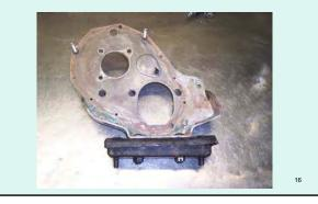
When a full pressure engine is mounted in a 1937 – 1951 passenger car, the standard 1935 – 1951 passenger front mounts can be used.
